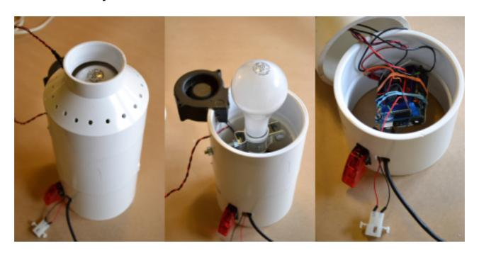
The temperature is monitored using a thermistor - basically a resistor that decreases resistance the hotter it
