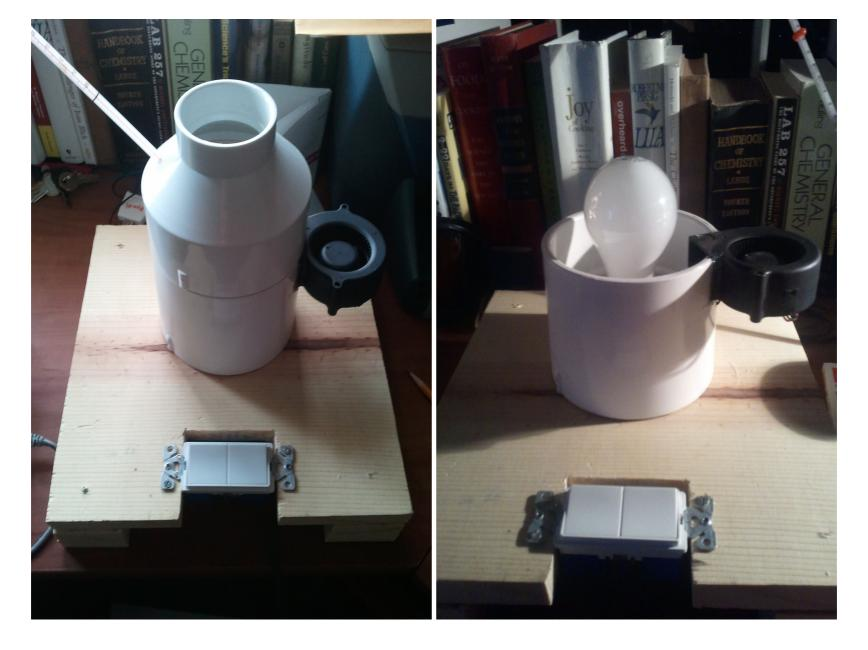
Instead of the switches pictured above, the unit is now controlled by an Arduino Uno, <u>Code Available Here</u>. It uses a thermistor (a resistor that allows more current to flow the more heat is available) to monitor the temperature of the samples. Here's the schematic:
